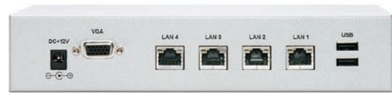
C•CURE 9000 SiteServer rear view showing network connections
